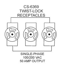
Figure 10. 100/100V Twist-Lock Auxiliary Receptacles Each auxilliary receptacle is protected by a 50 amp circuit breaker. These breakers are located directly above the GFCI receptacles. Remember the load output (current) on all three receptacles is dependent on the load requirements of the *Output Terminal Lugs*.
